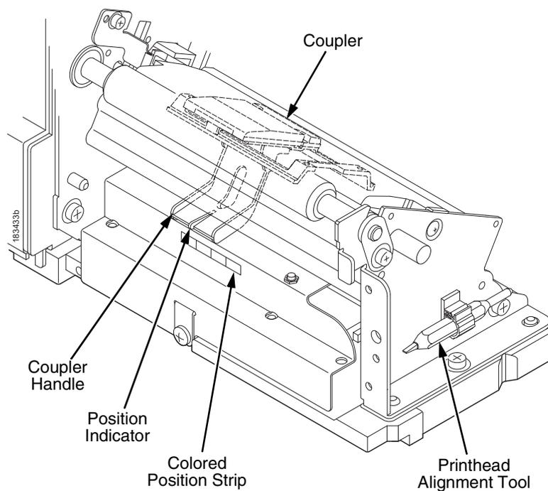
**NOTE:** To eliminate flexing of the coupler handle, use the printhead alignment tool (or a pencil or pen) to push against the side of the handle in the direction you need.
