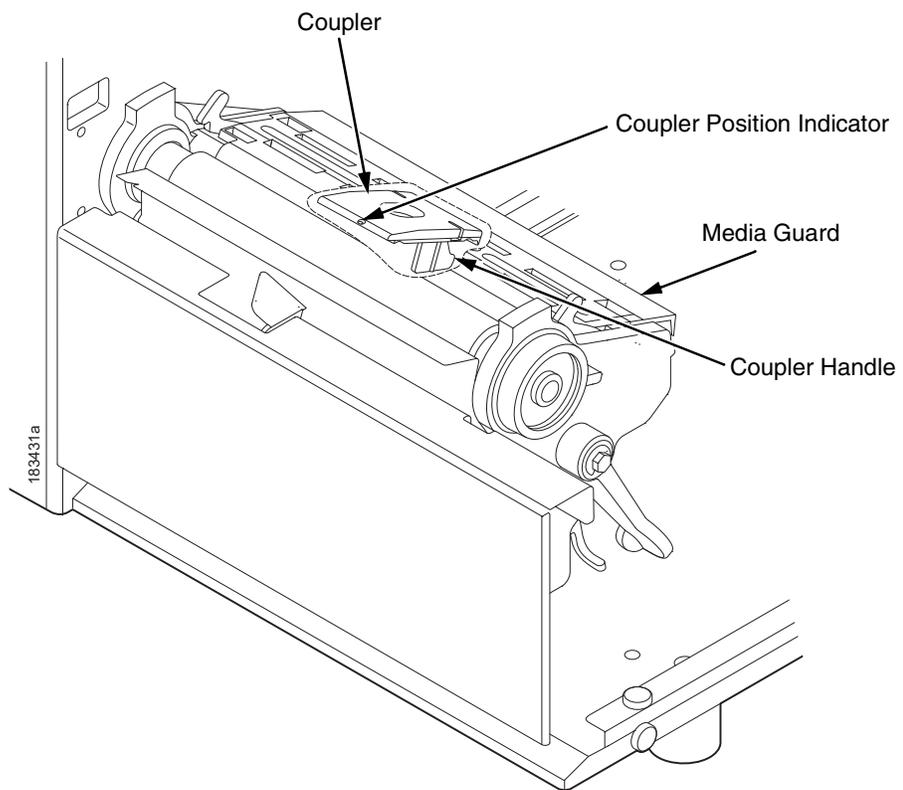
Reach under the media guard to grasp the coupler handle. Slide the coupler until the correct color displays in the coupler position indicator.
