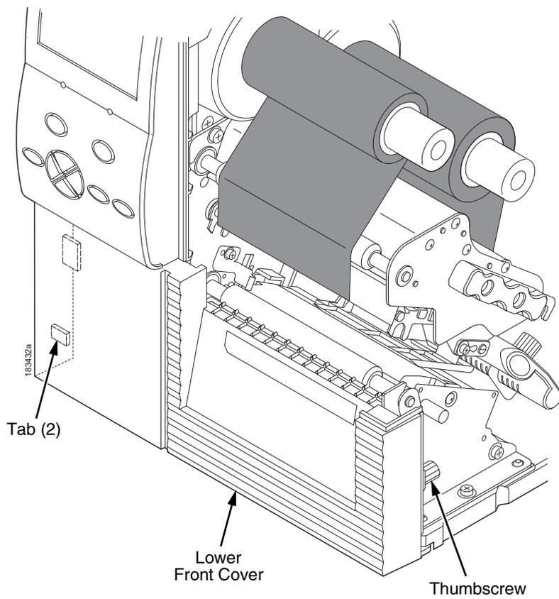
Remove the thumbscrew that secures the lower front cover to the printer. Slide the cover to the left to remove it.
